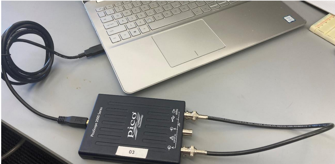
Figure 1. Connections for Generating a waveform and measuring it directly. The output waveform (AWG) is connected directly to input chan A with a coax cable. The picoscope is connected to the laptop via USB.
