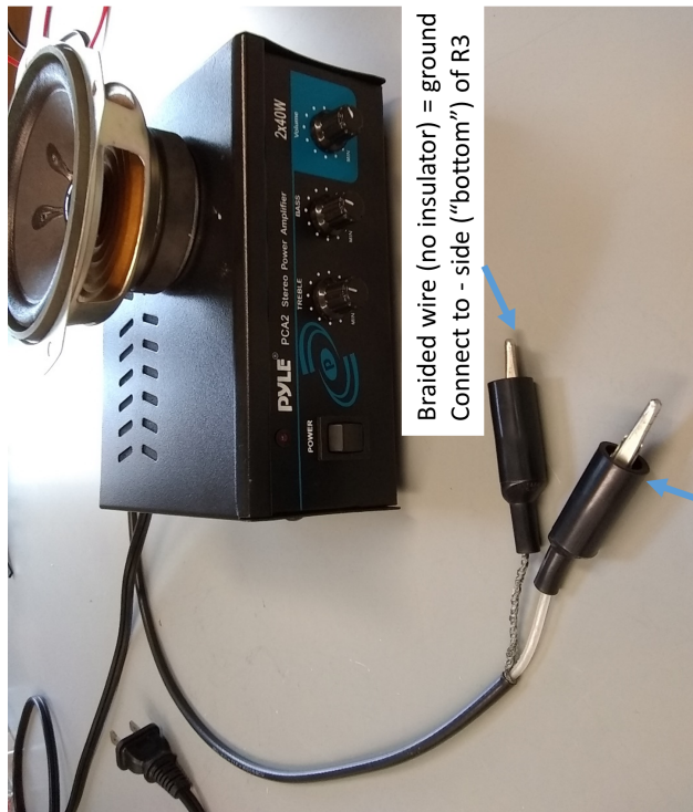
Figure 5: Connecting output of circuit/breadboard to audio amp and speaker
