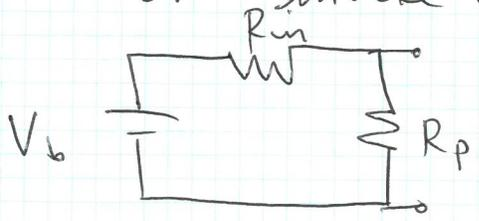
$$V_{Rp} = V_b \left( \frac{R_p}{R_{in} + R_p} \right) = \frac{R_1}{4}$$
