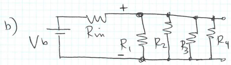
~~This~~ This configuration, all 4 motors plug directly into the power supply (NiMH battery). Think about the + and - terminals of the battery and where they line on the diagram.
