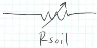
This is a variable resistor depending on hydration of soil.
