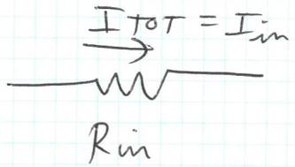
$$V_{in} = I_{in} R_{in} = I_{TOT} R_{in}$$
