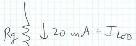
$I_{R_g} = 20mA$  . all current flow through LED must flow  $R_g$  . It is a series combo LED- $R_g$ !
