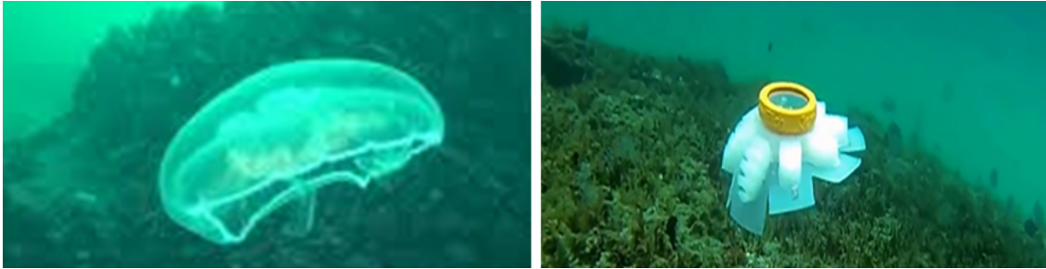
(a) A. aurita and bioinspired jellyfish robot patrolling coral reef
