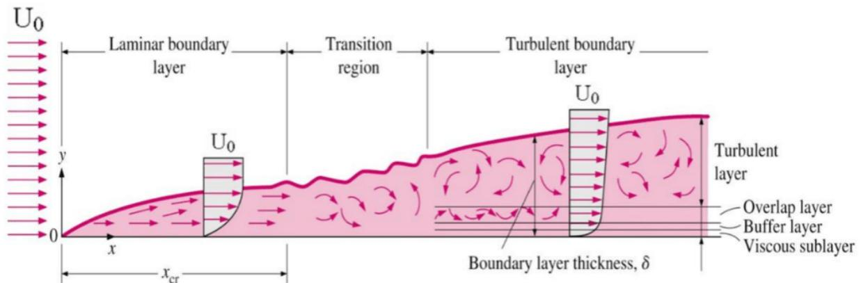
Figure 2: Boundary Layer Transition from Laminar to Turbulent Flow. Image credit: <https://www.nuclear-power.net/nuclear-engineering/fluid-dynamics/boundary-layer/>
