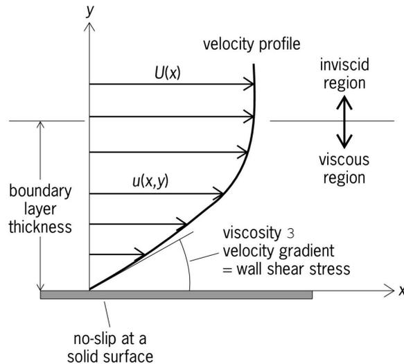
Figure 3: Velocity profile of boundary layer. Image credit:<https://encyclopedia2.thefreedictionary.com/boundary-layer+flow>
