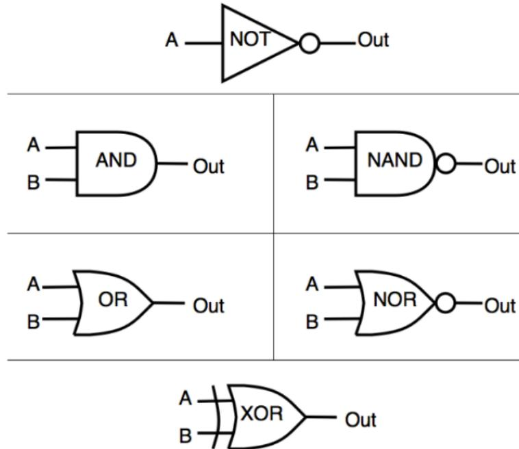
Figure 1. Logic Gate Symbols. The happy family of the 6 standard logic gates. Note the flat vs. curved back differentiating AND and OR. Also note the 'bubbles' indicate inverting logic—e.g. AND vs. NAND.
