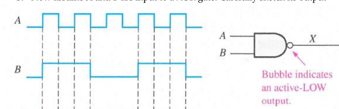
Figure 2. Digital pulse inputs to a logic gate. The regular period of each "clock cycle" is indicated by dotted lines. Image credit: Floyd, Digital Fundamentals 11ed, Pearson publishing
