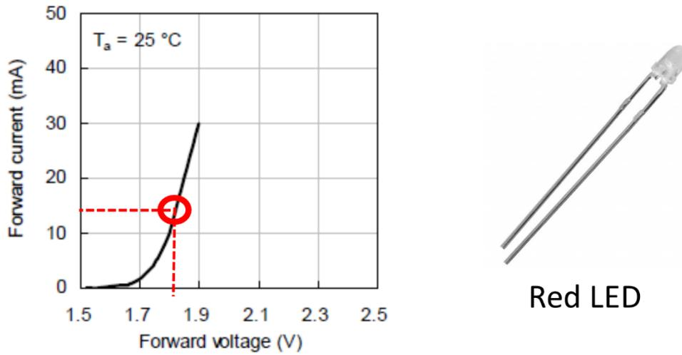
Figure 3. Red LED voltage-current characteristic curve (from the manufacturer datasheet). The device will flow about 15 mA when there is about 1.8V across the LED. When driven by a digital output of 3.3V, we need to dissipate  $3.3 - 1.8V = 1.5V$  elsewhere. This is the job of the current limiting resistor. Without, we would apply 3.3V across the red LED. Follow the exponential curve in your mind's eye to 3.3V—how much current would flow? LOTS, possibly burning out the LED.
