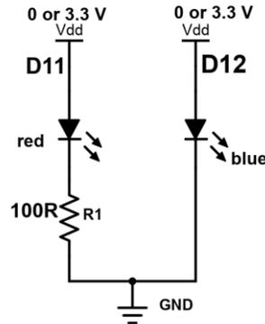
Figure 1. Circuit schematic for interfacing LEDs to Adafruit feather digital outputs that toggle LEDs on and off. The voltage of a digital outputs is 0V in the LOW state and 3.3V in the HIGH state. Note the red LED uses a current limiting resistor of approximately 100 Ohms; the blue LED requires no current limiting resistor in this case.
