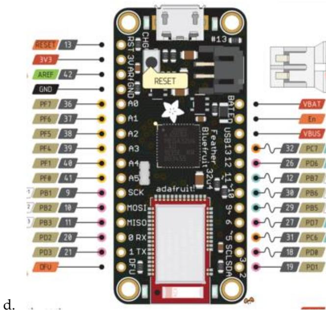
Figure 1. Adafruit feather 32u4 BLE pinout. Image credit: [https://cdn-learn.adafruit.com/assets/assets/000/046/242/large1024/adafruit\\_products\\_Feather\\_32u4\\_Bluefruit\\_v2.3-1.png?1504885170](https://cdn-learn.adafruit.com/assets/assets/000/046/242/large1024/adafruit_products_Feather_32u4_Bluefruit_v2.3-1.png?1504885170)
