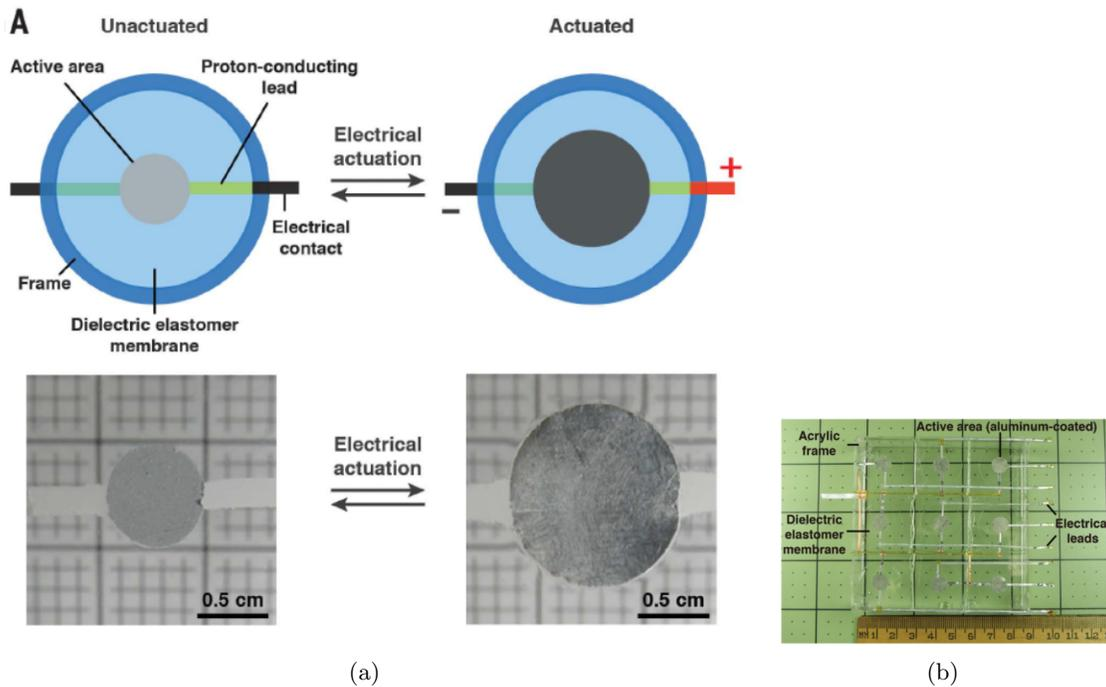
Figure 1: (a): Dielectric Elastomer IR reflecting “chromatophore” by Xu et al. (b):The actual bioinspired system on a lab bench. Science, 2018, 359:1495:1500.
