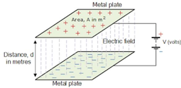
Figure 2: Charged capacitor model. The force generated by the charged plates squeezes (strains) the dielectric elastomer, causing the chromatophore to expand. Discharging the plates lets the chromatophore relax back to a smaller radius.
