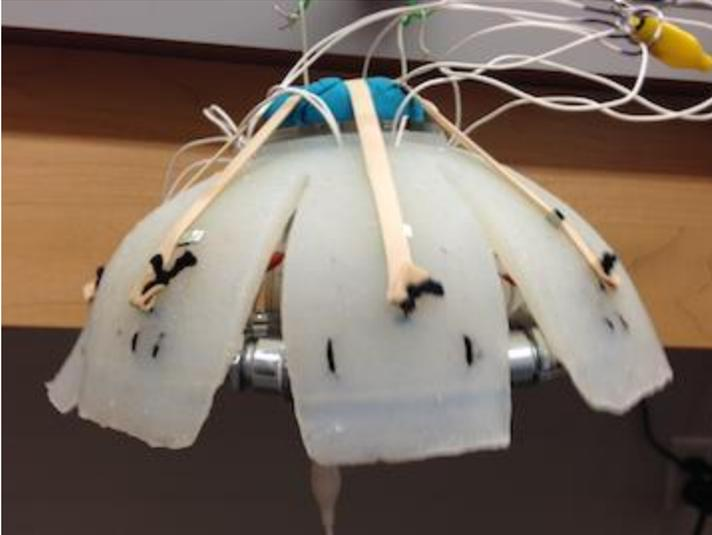
**Figure 9:** Our final jellyfish model during contraction with elastic recoil mechanism and solenoids tied underneath the bell.
