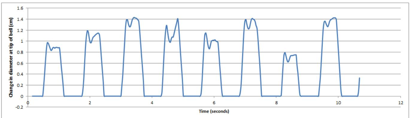
**Figure 12:** Graph of the change in bell diameter during out of water contractions at about 0.8 Hz with a duty cycle of 28% and a power consumption of approximately 78 Watts. The data has been smoothed with a 5-point moving average and normalized to zero for data points correlated to the relaxed state.
