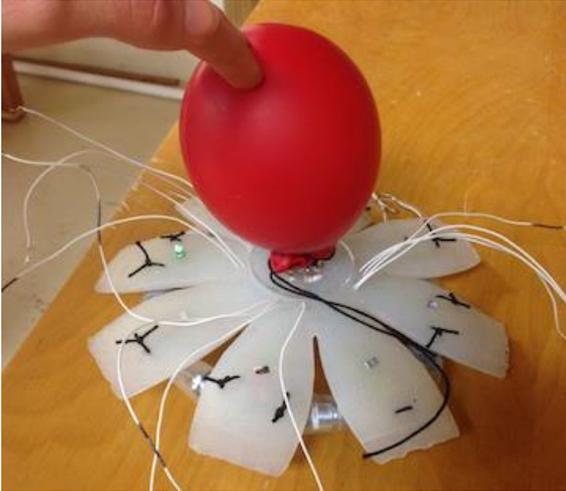
**Figure 14:** Image of the balloon buoyancy method. A balloon with a radius of 3.5 cm was closely attached to the top of the bell via a slip knot.
