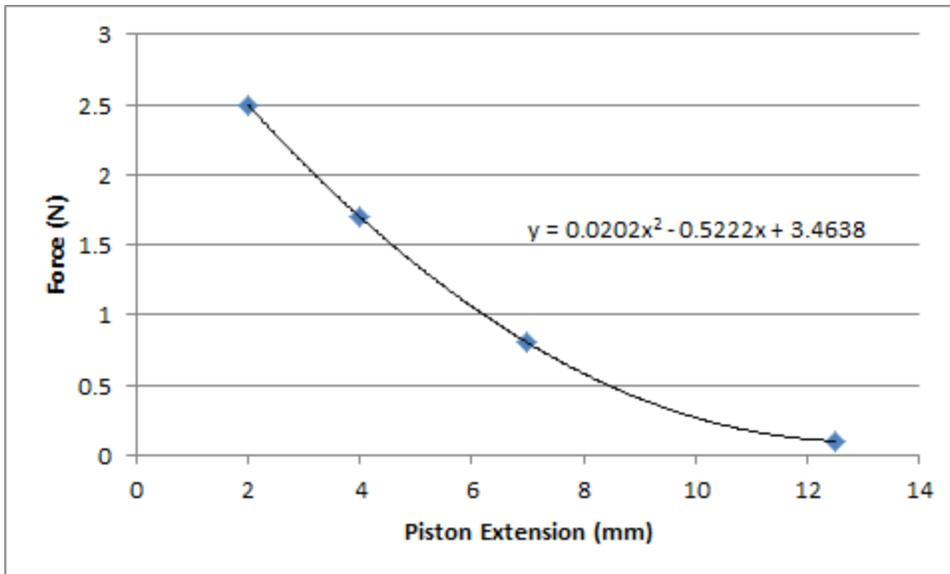
**Figure 10:** Force generated in a single solenoid operating with 2 Amperes (19.6 Watts) for different piston extensions. This serves to demonstrate the expected force in the solenoids and depict the decrease in force as the piston moves farther from the magnetic field.
