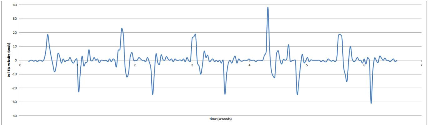
**Figure 13:** Graph of the bell tip velocity in air at about 0.8 Hz with a duty cycle of 28% and a power consumption of approximately 78 Watts. It is expected that the contraction velocity will be smoothed and much reduced in water.
