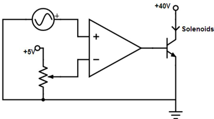
**Figure 8:** Circuit diagram of the driver for the solenoid actuator. A sinusoidal signal is transformed into a square wave by a comparator. The duty cycle is set by the voltage offset of the sine wave and the frequency of contraction is set on the function generator. A TIP 120 transistor was driven by the resulting square wave to allow high current to pass through the solenoids.
