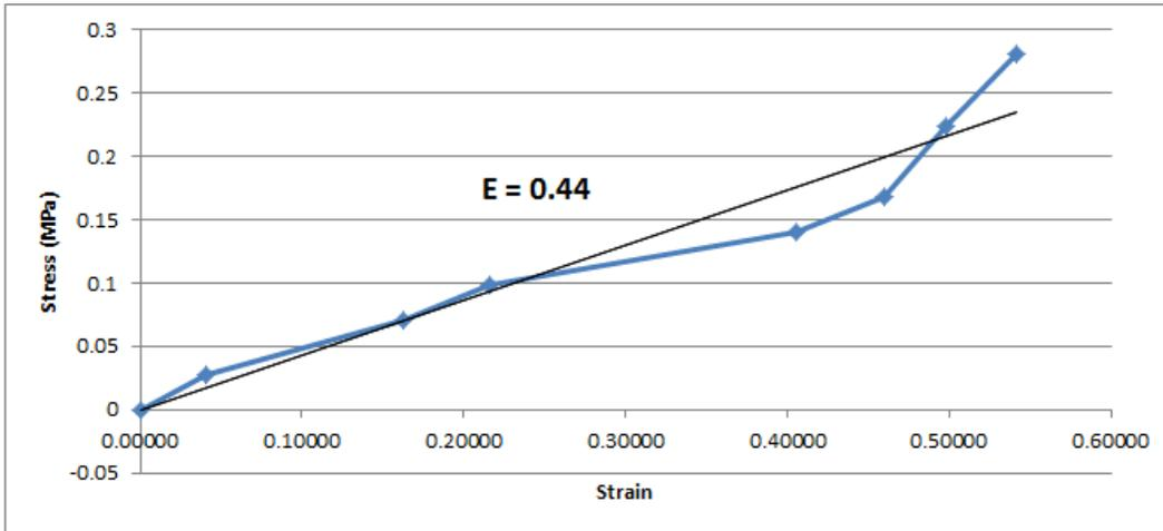
**Figure 3:** Stress-strain curve for a shore hardness 10A silicone cube with a cross-sectional area of 1.85 cm. The modulus of elasticity was calculated to be  $0.44 \pm 0.1$  MPa. For design considerations, the modulus of elasticity was taken to be 0.54 MPa.
