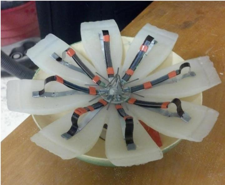
**Figure 6:** This depicts our recoil mechanism made out of aluminum and plastic. This was designed to assist the bell in relaxing after solenoid contraction. Further modifications would later be made to enhance our recoil mechanism.
