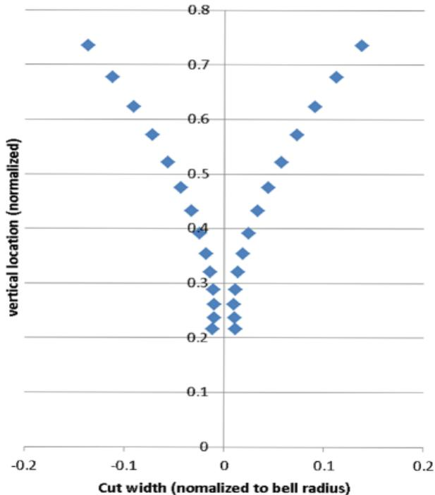
**Figure 5:** Graph of the points used to cut out bell slits in the CAD model in order to relieve stress that would have occurred due to reduction in circumference during contraction.
