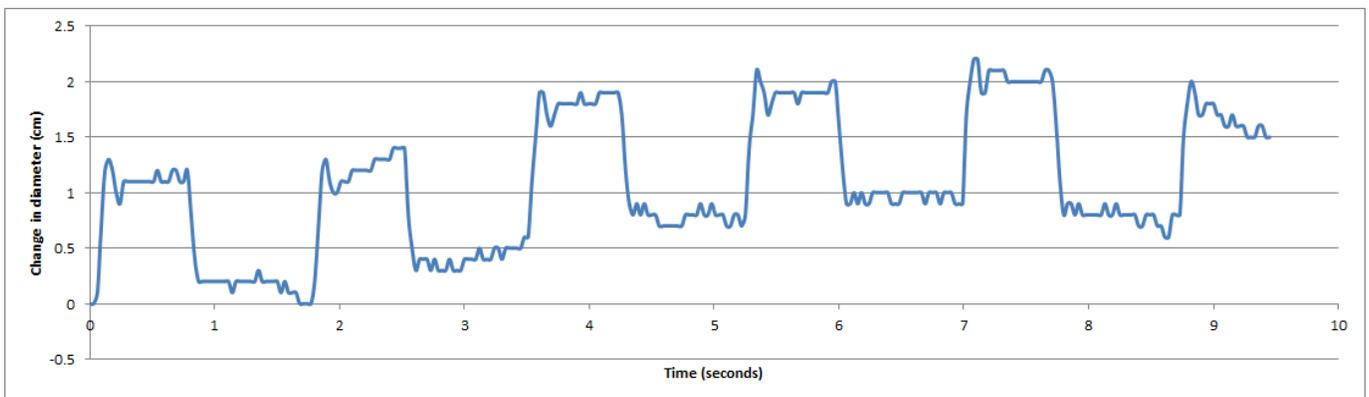
**Figure 11:** Graph of the change in bell diameter based on a preliminary video during out of water contractions for a duty cycle of 28% and a power consumption of 19.6 Watts. Note that the bell diameter decreases by 1 cm initially; however, the bell slumps since it is out of water. We anticipate that in water a 2 cm contraction could be achieved.
