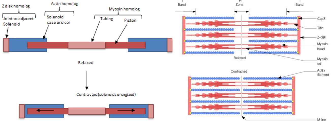
**Figure 1:** Comparison of the solenoid-based muscle with the microscopic muscular structure showing homologous components, the modularity and scalability is apparent is its conformity to the muscle architecture. (image on right from: <http://en.wikipedia.org/wiki/File:Sarcomere.svg>)
