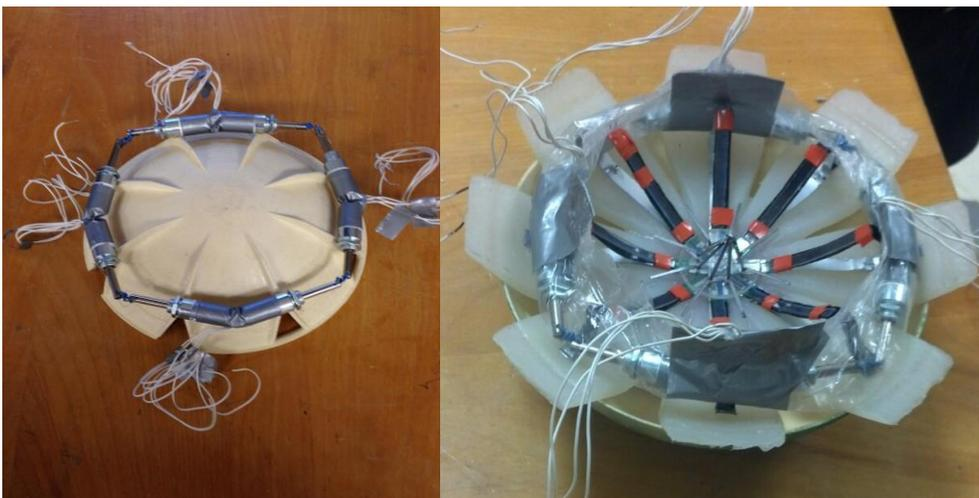
**Figure 7:** The left image depicts our circular actuator assembled using duct tape and thin wire. This displays the rough shape of our circular actuators and the rough positioning of the solenoids on the jellyfish bell. The right image shows our final waterproofing attempt made from polypropylene Ziploc bags, duct tape, and Liquid Nails.
