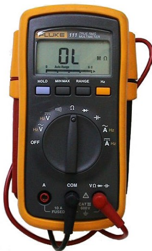
Figure 3: Meet your new friend in Circuit lab: the Fluke multi-meter. Note: red probe plugged into the right contact is required to measure voltage, resistance, and capacitance. To measure current, the red probe must be plugged into the contact labeled “A” (for Amperes).
