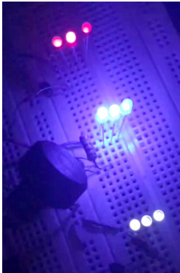
Figure 6: Illustration of 3 sets of illuminated LEDs synced to audio. Evidently, the bass, mids and treble channels were all outputting a relatively high (suprathreshold) level of energy at the moment this frame was captured. The potentiometer control knob is visible at bottom left. The current limiting resistor is visible for the bank of blue LEDs. Image courtesy of Chris Cotton, Circuits alumni fall 2017.
