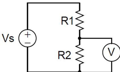
Figure 1. Basic voltage divider circuit
