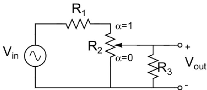
We measured the voltage output, which can be assumed to be proportional to audible volume.
