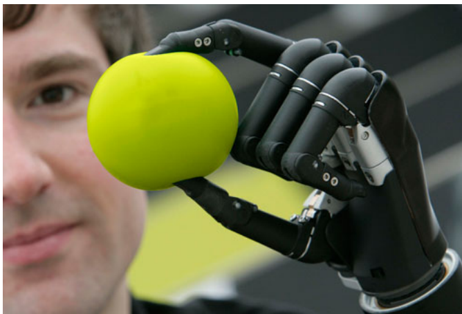
Figure 2: Touch Bionics iLimb Ultra. Dexterity is sufficient to squish a foam ball. The motion/grip of the prosthetic hand is driven by the EMG measured on the existing part of the amputee’s forearm. Image credit: http://www.touchbionics.com/products/active-prostheses/i-limb-ultra
