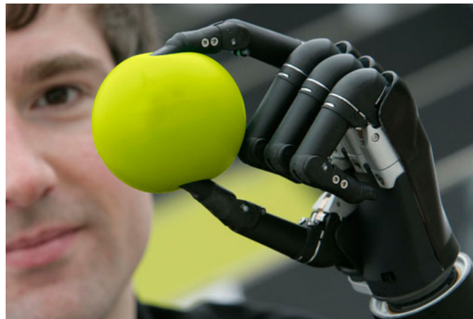
Figure 1: Touch Bionics iLimb Ultra. Dexterity is sufficient to squish a foam ball. The motion/grip of the prosthetic hand is driven by the EMG measured on the existing part of the amputee's forearm. Image credit: http://www.touchbionics.com/products/active-prostheses/i-limb-ultra
